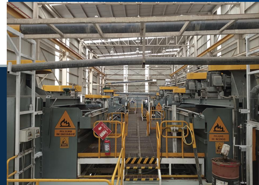
Flotation area: Wenco cells and two concentrate filters
